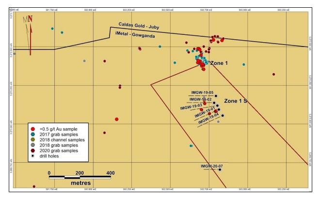
An initial diamond drilling program of 6 holes totaling 2010 metre was completed in February 2019, with 5 of the six holes testing Zone 1 south. A  $7^{th}$  hole was completed further to the south along Zone 1 South in February 2020. The drill hole details are shown in Table 3.
